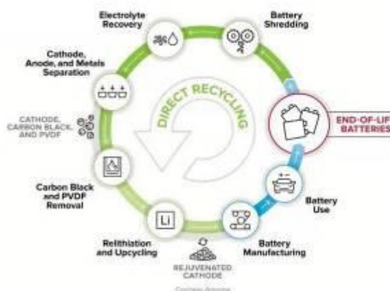
Typical Direct Recycling Process Flow
